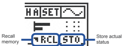
Fig 5-08, Channel status memory field
