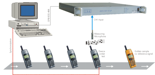
Fig.4 Signal verification setup
